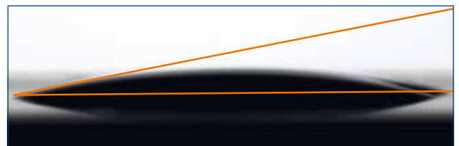
V-Posil Light Fast / V-Posil X-Light Fast / V-Posil Mono Fast – small contact angle of < 10^\circ
